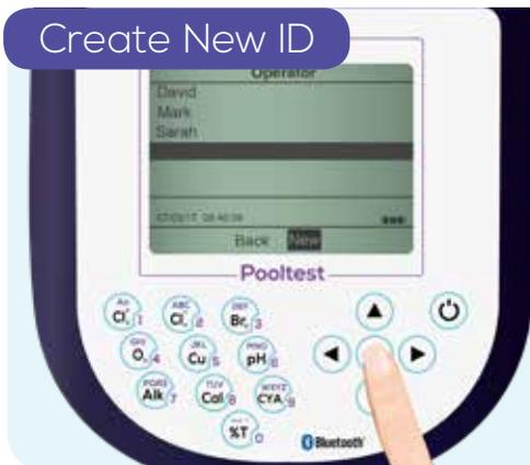
To create a new Operator ID or Sample ID, scroll to the bottom of the list, then select 'New' to create an ID.
