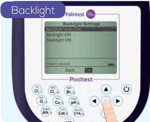
The instrument display features a high intensity backlight for use in low light conditions. To change the backlight settings, from the main menu select 'System mode' then 'Backlight'. Highlight the preferred option and press OK.
