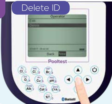
To delete an Operator ID or Sample ID, highlight the option, and select 'Delete'.
