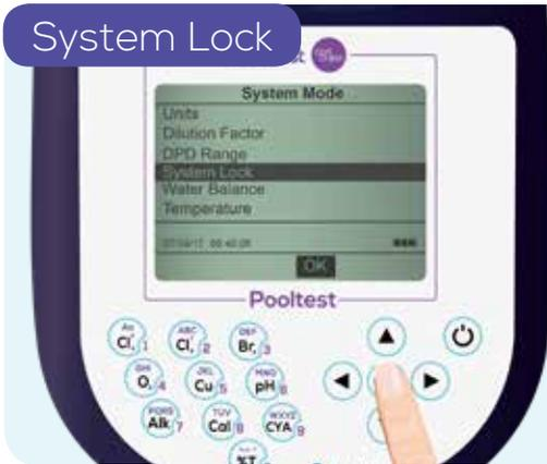
The system settings can be locked to prevent changes. From the main menu, select 'System Mode', then 'System Lock'. To lock or unlock the instrument enter the code 6812. To change this code, contact Palintest.
