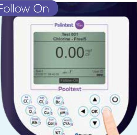
Refer to the test method to see if this is required. If a follow-on test is available, it will appear in the bottom menu. Select if required.
