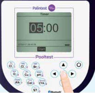
A timer can be set after the blanking process. Refer to the test method to see if this is required. The development time for the test will automatically appear. This can be modified using the arrow keys. Press start to set timer running.
