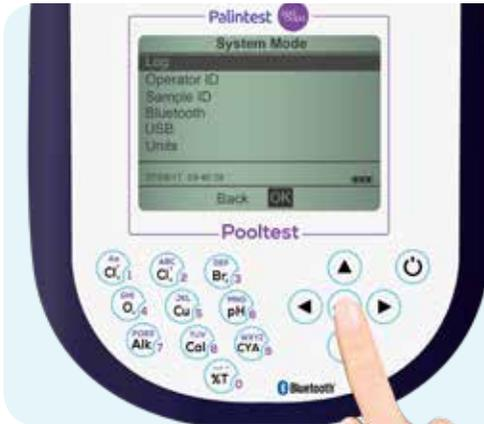
To access Operator ID or Sample ID from the main menu select 'System Mode' then 'Operator ID' or 'Sample ID'.
