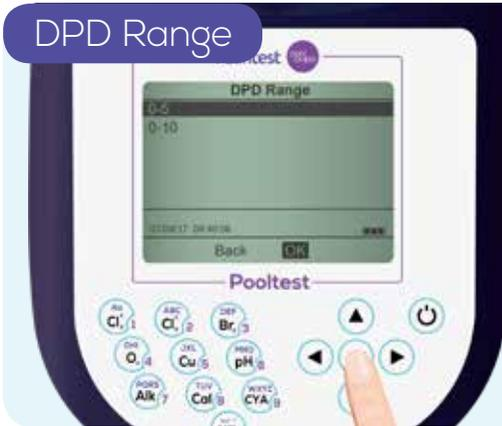
There is a choice of two ranges for the DPD test for Free and Total Chlorine. See Test Instructions to ensure that range selected matches the reagents being used.
