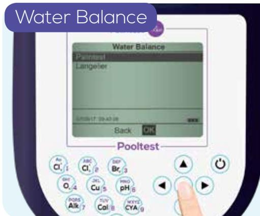
Water Balance can be set to use the Palintest Scale or Langelier Index. Select the preferred option and press OK
