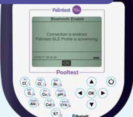
Select Bluetooth Communications ON. Enable Bluetooth on a mobile device and pair the devices from within the Aqua Pal App.
