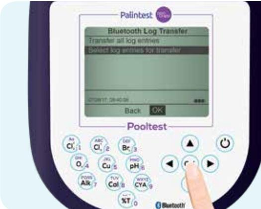
To transfer a specific log file, highlight 'Select log entries for transfer'. Use the up and down arrows to find the correct log entry and select OK. 'Log transfer complete' will display when the process is complete.
