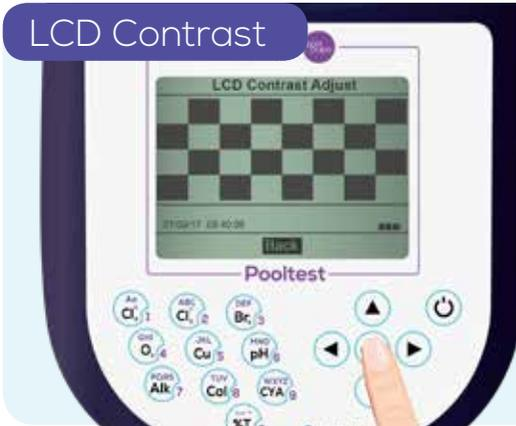
From the main menu select 'System mode' then 'LCD Contrast'. The LCD screen contrast can be manually adjusted. Use the up/down buttons to adjust the contrast until the alternating shapes are clearly visible and press 'Save'.
