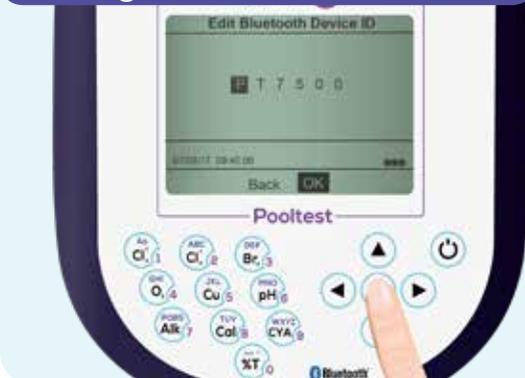
To change the Bluetooth Device ID, Select 'Bluetooth Device ID' and change as required.
