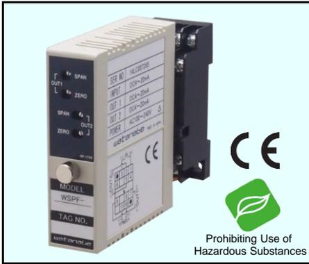
This compact plug-in type converter (isolator) provides 2 signal outputs which are mutually isolated between input, output and power-supply. It amplifies and converts various kinds of signal with isolation to use in the integrated instrumental control system. It is highly effective as noise countermeasures.
