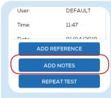
Press ADD NOTES to type information about the test using the on-screen keyboard. Maximum of 48 characters. After a failed test, it is recommended to write an explanatory note or explain the corrective actions taken, as the information will be stored alongside the test in memory.
