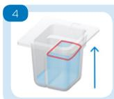
Fill the right side of the vessel to the line. If there is excess sample, it will pour into the left side of the vessel. Do not overfill both sides or water can splash onto the sensor contacts and interfere with the test.
