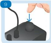
Press the start button on the pump to begin degassing the chlorine dioxide from the sample.
