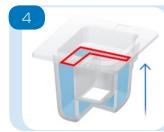
Fill the L-shaped vessel to the line. This is so that the temperature probe is in contact with sample for temperature compensation.
