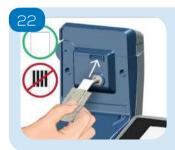
Hold the final CDX sensor through the foil packet only, with the white side facing up. Slide it all the way in, until the end stops against the back of the slot.
