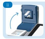
While the degasser is running, prepare for the next sensor test. Open the lid, remove the sensor, and discard the old sample.
