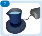
During the one minute electrochemical measurement period, set up the degasser as shown. Ensure the two plastic halves of the degasser are properly connected. Ensure the filter is installed correctly.
