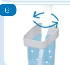
Add one Soluprep SP-A tablet into the disposable vessel. Crush and stir using the crushing rod until the tablet is fully dissolved.
