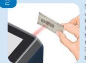
Scan the sensor barcode using the barcode scanner. Hold the barcode about 12cm (5in) from the instrument. Align the red dot with the center of the barcode. When the scan is complete, the instrument proceeds to the next screen.
