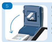
Pull the foil off the sensor. Close the arm. The test will start automatically.
