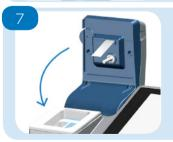
Pull the foil off the sensor. Close the arm. The test will start automatically. Wait three minutes (lead) or 5 minutes (cadmium) while the instrument performs the electrochemical measurement
