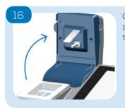
Open the arm, discard the sensor. KEEP the sample from the previous test.
