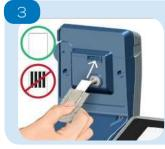
Hold the sensor through the foil packet only, with the white side facing up. Slide it all the way in, until the end stops against the back of the slot.
