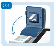
Pull the foil off the sensor. Close the arm. The test will start automatically.
