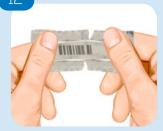
Tear each side of the second CDX sensor packet, then twist and tear the short side from the packet, revealing the sensor tracks. Do not touch the dosed half of the sensor.
