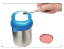
20 Starting at the far edge of the petri dish, use a rolling motion to place the membrane filter on top of the absorbent pad. This will prevent air being trapped between the pad and membrane filter.
