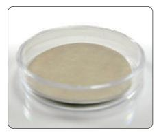
**NutriDisks** are the option most commonly used with the Wagtech Test kits. **NutriDisks** are larger than the standard aluminium petri dishes supplied in the kit but are still designed to fit into the standard petri dish rack. This allows up to 7 **NutriDisks** to be incubated at the same time.
