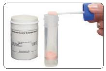
Fill the MMD with sterilised water to the lower lip and screw the lid on tightly.
