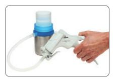
12 When all of the sample has been filtered, detach the vacuum pump and remove the filter funnel from the rubber base. The membrane filter is now ready to be removed and placed in the petri dish containing the absorbent pad and growth media.
