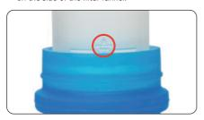
8 Pour the water sample into the filter funnel up to the 100ml graduation (or less if using a smaller sample).
