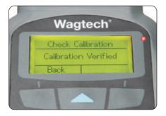
The Check Calibration function provides a simple electronic check that both thermistors are reading the same temperature as each other within a specified tolerance. If the comparison is out of range the display will show **Error 107: Validation**.
