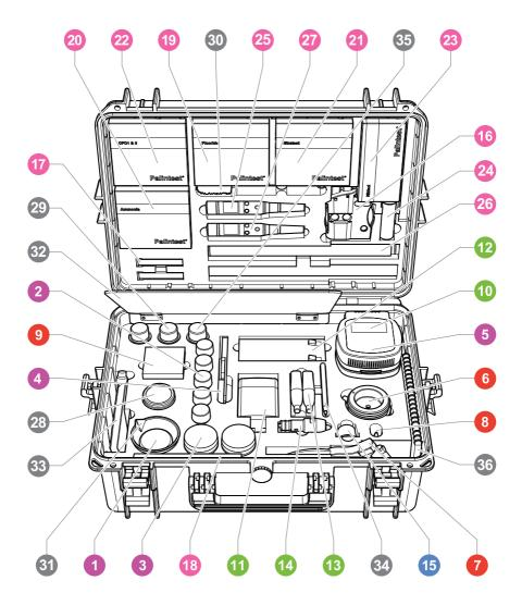
**Fig 1. Potakit**<sup>™</sup> **+** Water test kit opened to show contents. Coloured circles indicate the chapter colour in which their use is explained.
