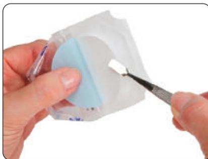
**4** Peel back the transparent outer wrapper and use the sterile forceps to separate the white, gridded membrane filter from its blue backing paper and remove from the outer wrapper. Only ever grip the membrane filters at their edge.
