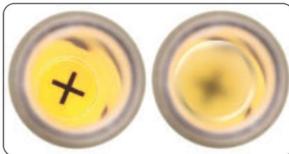
Read the turbidity value from the level of sample against the scale etched on the tube. Estimate the result if the level is between values.
