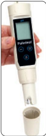
The upper display will show the actual reading, the lower display will show the buffer value. Insert the probe into 2-3cm of buffer solution and stir/rotate gently. The protective cap can be used to hold the buffer. Allow the reading to stabilise and press **HOLD/ENT** to confirm the value. Rinse the electrode with clean water and repeat as required with additional buffers. Press **CAL** to exit calibration mode at any point.
