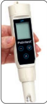
Note the reading or press **HOLD/ENT** to store the reading on the display. Press **HOLD/ENT** to return the display to normal mode. After measurement rinse the electrode with clean water. Store the electrode with a moist piece of paper in the protective cap if possible to avoid the electrode drying out.
