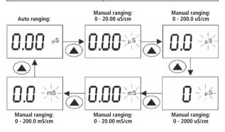
**NOTE:** If the value of the solution you are measuring is higher than the range selected [□¬] (over range) will appear. Press ▲ to select a measurable range. The meter resets to Auto-ranging function once it is turned off. You will have reset the manual ranging function each time you turn the meter off.
