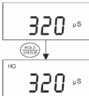
**NOTE:** The meter will shut off automatically after 20 minutes of the last key press. If the meter is shut off either automatically or manually, the HOLD value will be lost.
