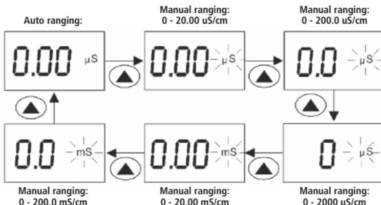
**NOTE:** If the value of the solution you are measuring is higher than the range selected [OL] (over range) will appear. Press ▲ to select a measurable range. The meter resets to Auto-ranging function once it is turned off. You will have to reset the manual ranging function each time you turn the meter off.
