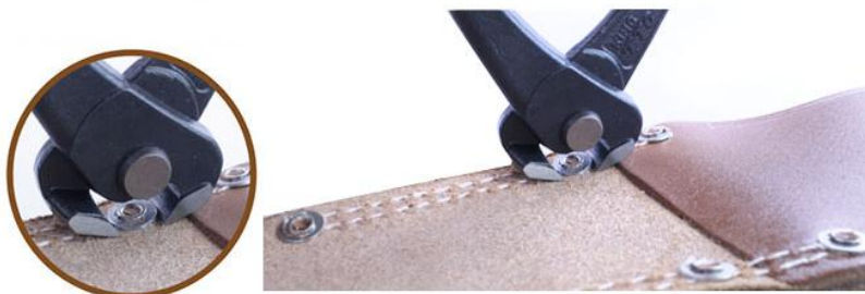
Removing metal parts.
