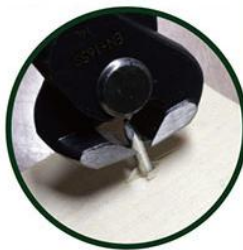
Cutting nails and pulling out.
