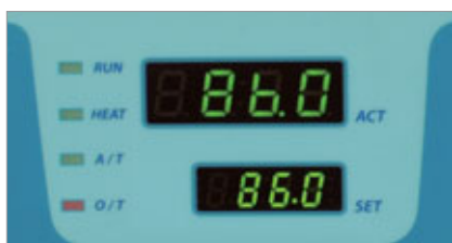
Simultaneously displays set temperature and actual temperature.
