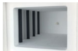
1500°C model (2-side exposed type heater)
