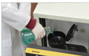
Wide inlet of waste liquid funnel.
