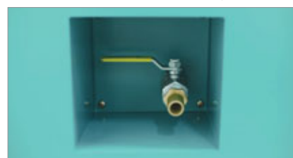
Spill drain port for clean internal management.
