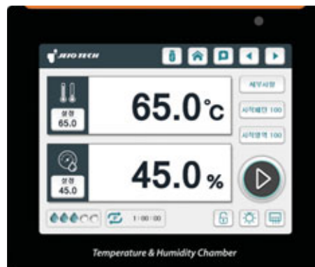
Large LCD touch screen controller (5.6 inches)
