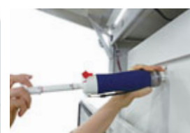
Checking filter saturation
