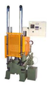
This machine is a compacting machine for plastic and rubber. The heat platen is heated electronically and pressure is applied with a manual oil pressure pump. The upper platen can be adjusted and fixed to the optimal position with a nut to provide great operability.
