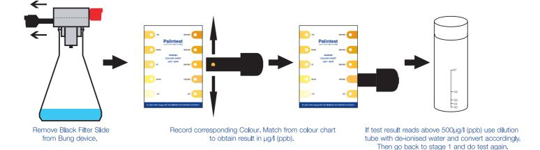
For Verification of readings less than 100µg/l (ppb)...
