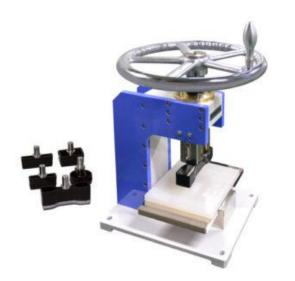
This device is used as a handle type cutting machine to prepare specimens of non rigid plastic, rubber sheet, etc. The device is assorted with a variety of cutters so that it enables to prepare dumbbell, ring, and angle type specimens.
