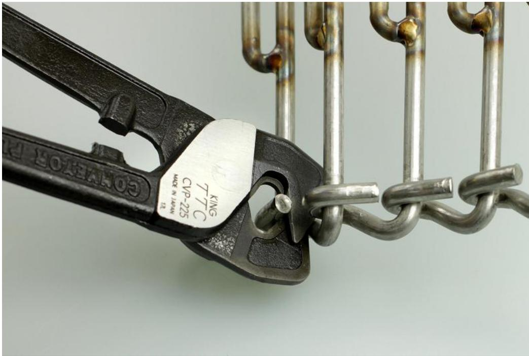
Opening : Insert the claws into the loop.
