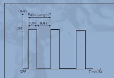
Controller Signal of Pulse Frequency Control
