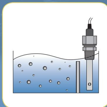
**Figure 5:** Submersible installation
