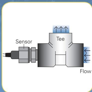
**Figure 4:** In-line installation
