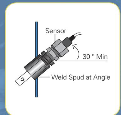
**Figure 6:** Angle mounting installation
