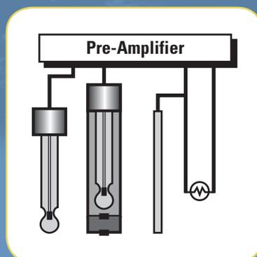
**Figure 2:** Differential electrode replaces porous reference electrode with a glass electrode
