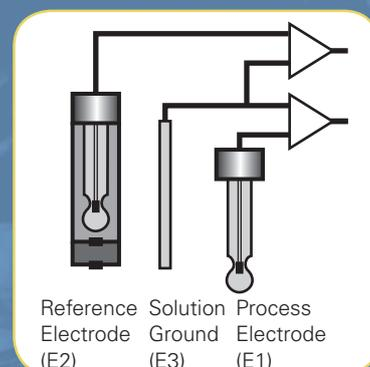
**Figure 3:** Individual liquid ground loop eliminates noises from ground loop potentials
