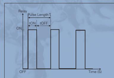
Controller Signal of Pulse Frequency Control
