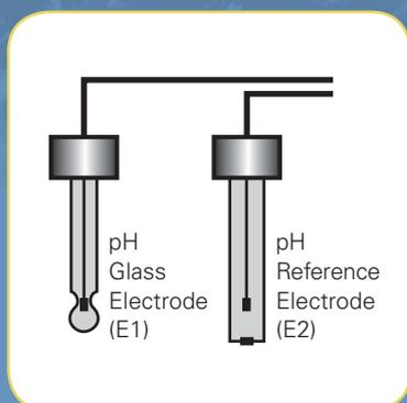
**Figure 1:** The conventional combination electrode is made up of a glass electrode and a reference electrode
