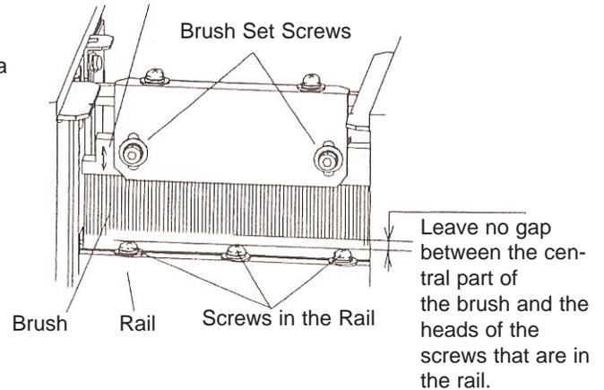
4. No adjustment is needed if there is no gap between the central part of the brush and the heads of the screws that are in the rail.
