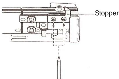
The stopper can move up and down, after you loosen two screw from the stopper
