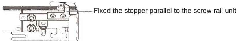
After adjusting the height of the screws, head fixed the stopper parallel to the screw rail unit with two screws.
