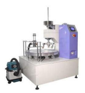
JIS-A1454, L1021-11, (L1023), L4406, DIN-54 342 This tester enables caster chair test for floor materials and floor cloth. By placing a caster chair that has prescript load to onto the continuously rotating circular specimen table, the operator is to evaluate the abrasion resistance of the test specimen by measuring the thickness of the test specimen.
