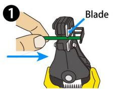
Insert wire into correspond hole on the blade.
