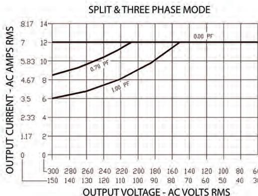
Short term overloads to 15 Amps are permitted. Operating time before thermal shutdown or circuit breaker trip varies from seconds to several minutes depending upon line and temperature conditions.
