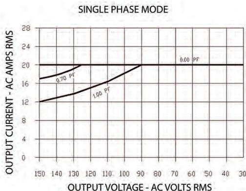
Short term overloads to 30 Amps are permitted. Operating time before thermal shutdown or circuit breaker trip varies from seconds to several minutes depending upon line and temperature conditions.
