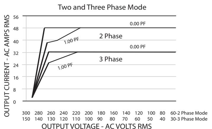
Short term overloads to 120A are permitted. Operating time before thermal shutdown or circuit breaker trip varies from seconds to several minutes depending upon line and temperature conditions.
