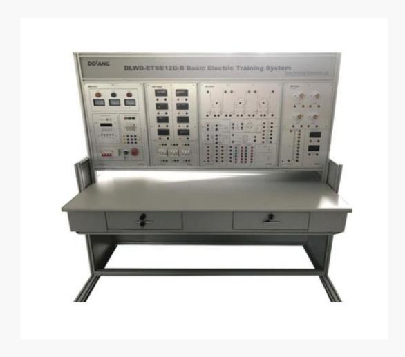
DLWD-ETBE12D-B basic electric training system provides a set of measuring instrument modules, rectifier, filter, adjustable resistor module, load module and so on. It is mainly used in basic electrical teaching experiments.
