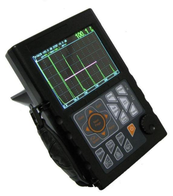
YFD300 Ultrasonic Flaw Detector Weld Testing Equipment
