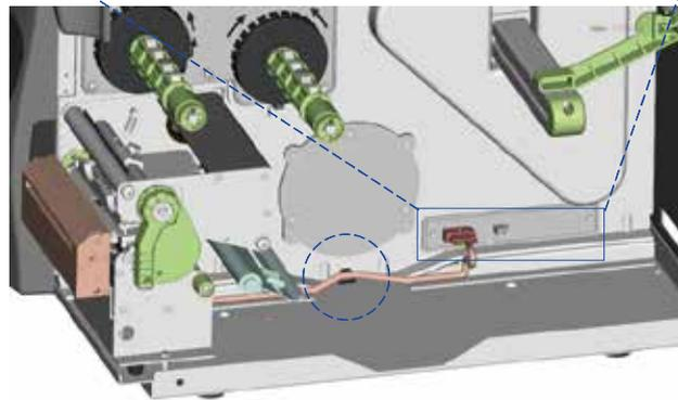
6. Place the cutter cover over the cutter module and secure it using the screw you removed from the lower cover plate.
