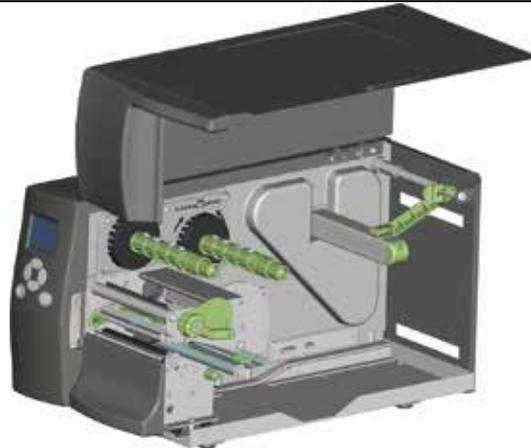
2. Pull out the print head release lever as shown in the illustration (1) and turn it anticlockwise to a top right position (2).
