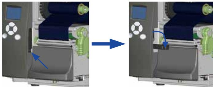
13. Close the printer cover to complete installation of the dispenser.
