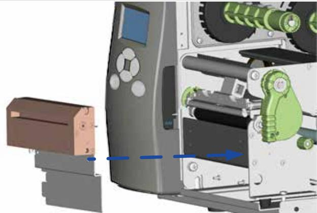
4. Connect the cutter cable connector to the cutter jack on the printer.
