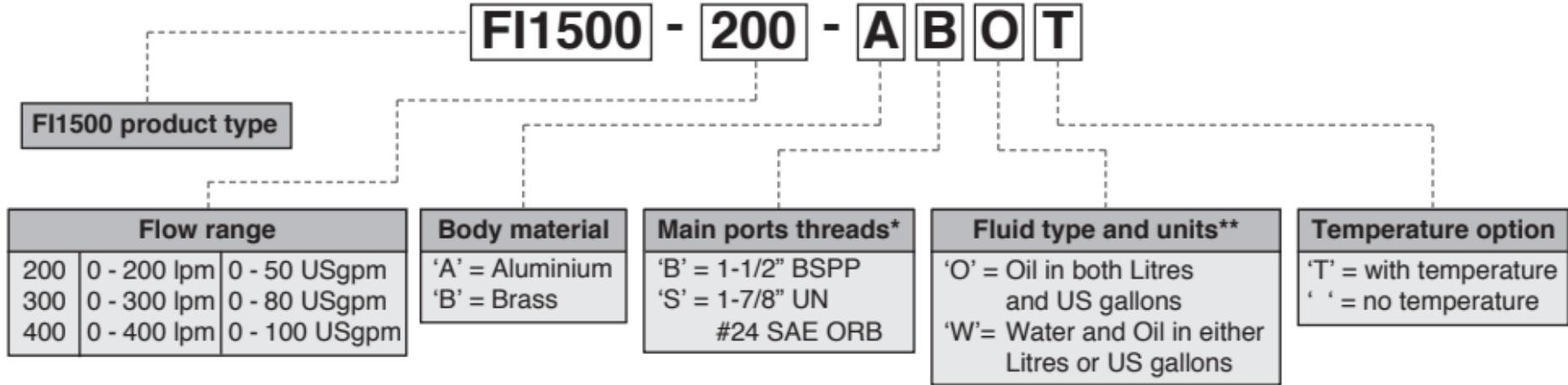
\* Pressure ports follows main port - 'B' main port - 1/4" BSPP pressure port
