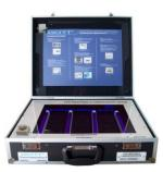
Illuminated Magnifier PCB Checker ...... 1 No. (Magnifies the job kept under it to 2 times its size, two and half inch area is magnified)
