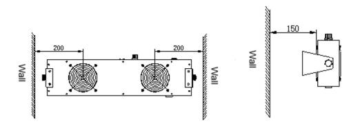
While using the ionizing air blower, the mounting bracket should be fixed on a solid and flat surface (such as a wall or a shelf) with screws
