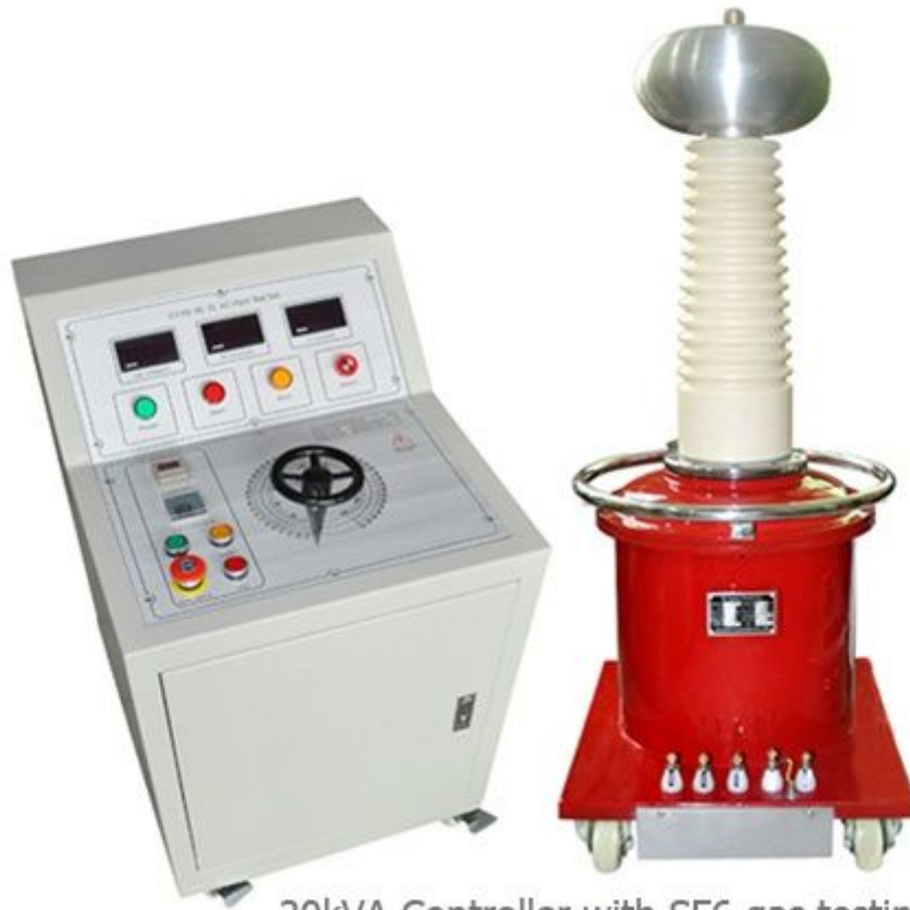
20kVA Controller with SF6 gas testing transformer
