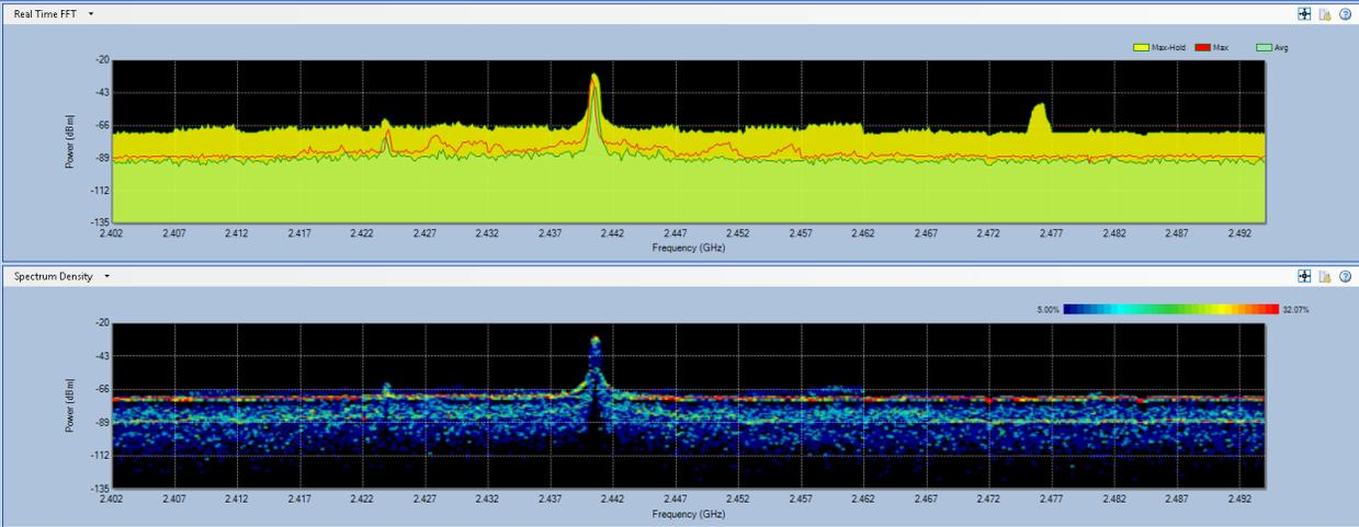
**RF Spectrum Pattern of a Narrowband Jammer**
