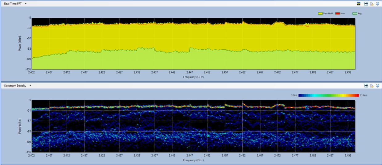
**RF Spectrum Pattern of an RF Jammer**
