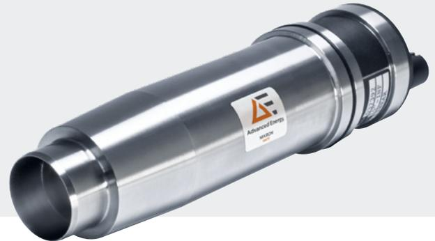
Completely self-contained, the Mikron® M67S infraducer can be used as true two-wire temperature transducer/transmitter which produces a standard 4 to 20 mA linear output. Powered by its current loop, each infraducer is completely compatible with any existing instrumentation for recording or process control.
