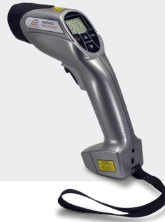
The Impac® IGA 15 plus infrared thermometers are high-quality, battery driven portables for non-contact temperature measurement. The instruments feature a built-in data logger (750 values), a laser targeting light, and a short exposure time. With the high-quality optics, accurate measurements of small objects can be made at a distance of 4 mm (1.25 mm with the close-up lens).
