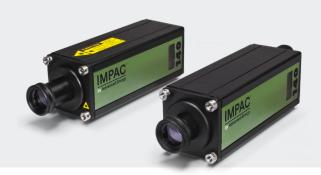
The Impac® IPE 140/45 is a special pyrometer for the temperature measurement of hot,  $CO_2$  containing combustion gas. The pyrometer is able to measure hot combustion gas (with typically approx. 10%  $CO_2$ ) with a thickness of 40 cm.
