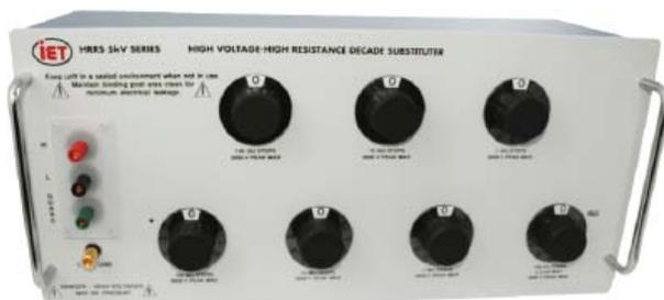
**Figure 1-1: Example of an HRRS-5kV unit with 7 decades**
