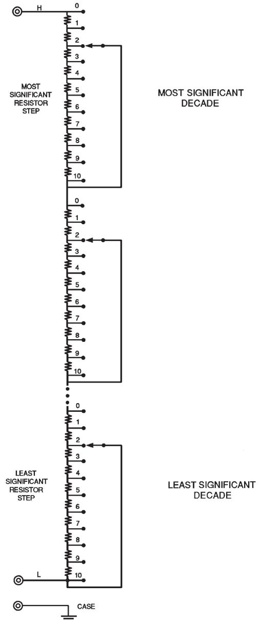
**Figure 4-1: HRRS 5kV and 10kV Series Schematic Diagram**
