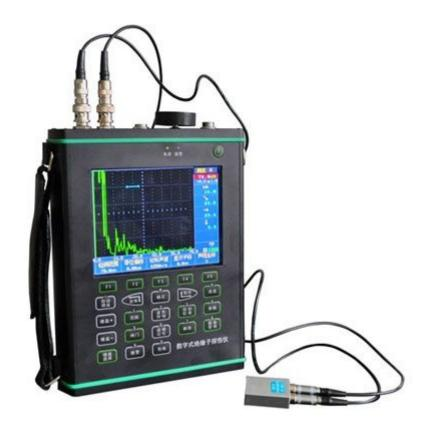
Ultrasonic Flaw Detector is a non-destructive testing device used for detecting internal mechanical damages for electrical equipment.
