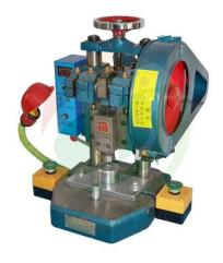
Automatic Coin Cell Crimper For Coin Cell
