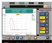
70Xi screen displays real-time test results and phase plot, showing temperature change and signal strength as test progresses. The graphic visual information helps users better understand anomalous behavior.
