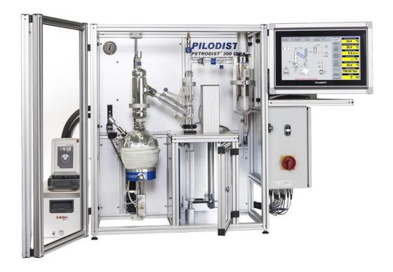
Processor controlled Crude oil distillation system according to ASTM D-1160. System for determination of boiling ranges of crude oil products under vacuum in fully automatic operation.
