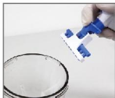
You can press the ejector bottom to eject tips.
