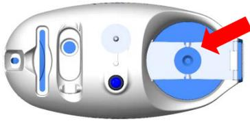
Confirm the centrifuge tube rack is stable by checking the positioning hole in the middle of the rack.
