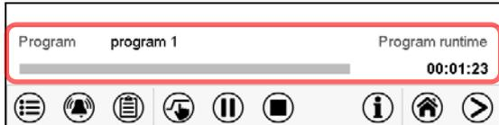
Normal display. Information on the bottom of the screen indicates the currently running program and the time already passed. The grey bar shows how much time of the whole time is elapsed. If program duration has been set to infinite, the grey bar is not displayed.
