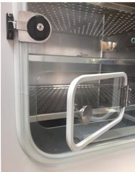
Figure 25: Glass door (detail, example door hinge on the right) with Quick sample access option
