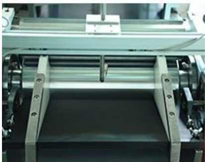
Slurry dam board and stirring paddle
