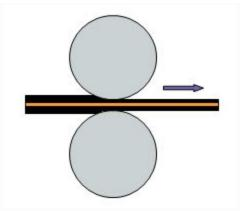
Battery electrode roll press process
