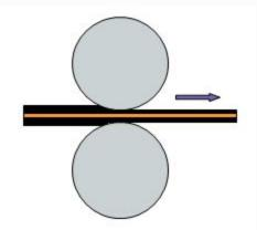
Battery electrode roll press process
