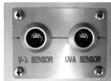
Figure 13: Lemo sockets to connect the light sensors
