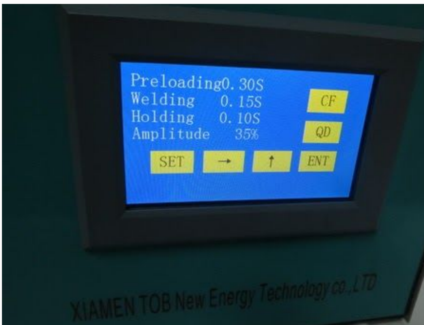
Touch-screen controller with setting parameters
