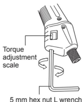
2. Turn the driver on and tighten a screw to check that the driver stops at a satisfactory level of tightness.
