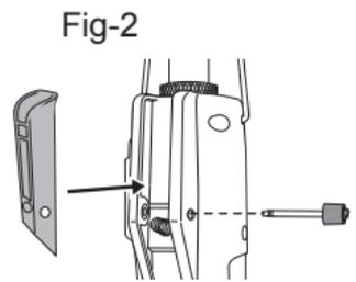
To convert the starting mechanism from lever-start to push-to-start, remove the hex head screw and switch lever, turn the switch lever upside-down and use the hex head screw to re-fasten the switch lever.
