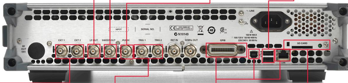
Sum external 1 and 2 inputs for composite analog modulation of AM or FM/PM, or digitally sum with multi-function generator Option 303.
