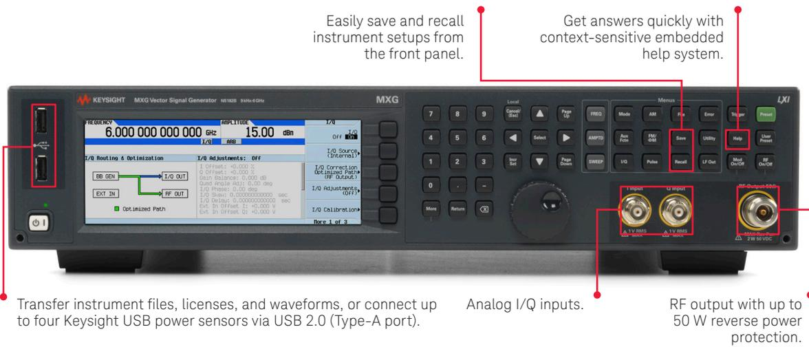
Easily save and recall instrument setups from the front panel.
