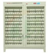
Mainly composed of a communication interface and a battery detection cabinet. The battery testing cabinet is composed of battery clamp and a plate body to placing fixture, a constant current constant voltage source, a registration control circuit, a sampling circuit, a single chip microcomputer and a control panel.
