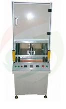
**1.Applicable to polymer battery core hot press.**
