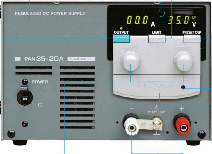
**Voltage and current preset variable resistors**
