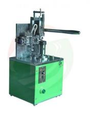
Aluminum Case Supercapacitor Grooving And Sealing Machine
